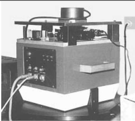
Figure 4. General view of the laser goniometer IUP-1L. The upper plate of the device supports a photoelectric angle encoder RON255 mounted ready for the calibration.
