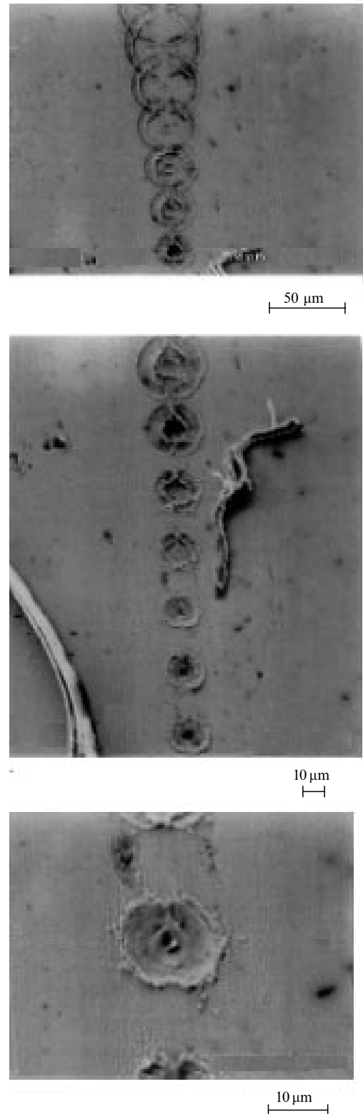
Figure 3. Ablation imprints on the brass target as it was moved from the mirror to the focus. Each imprint was produced by a single pulse of laser irradiation.
