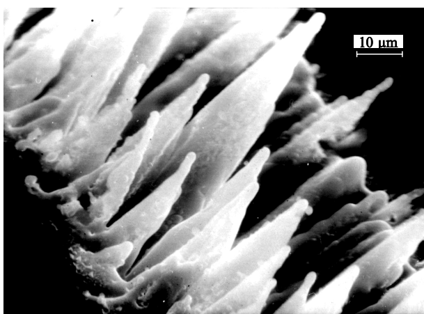
Figure 3. Microstructures growing upon oblique incidence of laser radiation on the silicon surface in vacuum at an angle of 60^\circ .
