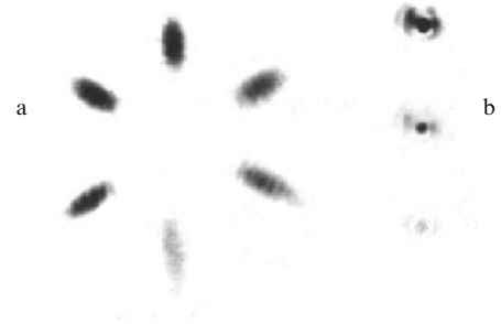
Figure 11. Image in the far-field radiation zone formed only by the PM of the TENOCOM system without compensation for the mutual tilt of subapertures (a) and by the entire TENOCOM system with the same PM (b); presented are three images detected with different attenuation.
