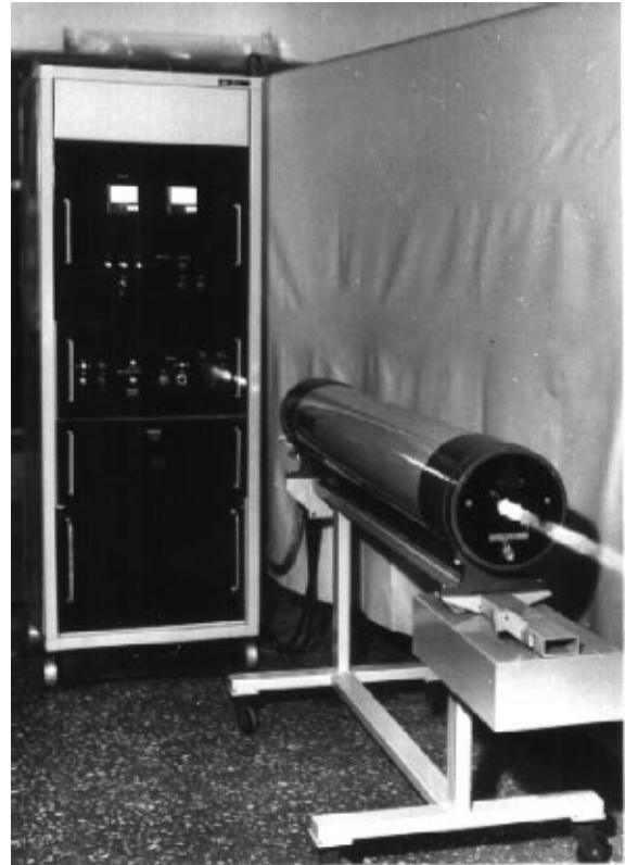
Figure 12. LGI-202 'Kurs' copper vapour laser.
