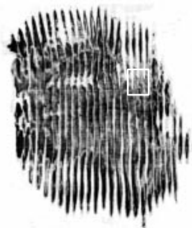
Figure 5. Interference pattern of the transverse shift of the laser beam. The frame in the pattern field indicates the position of a dislocation.
