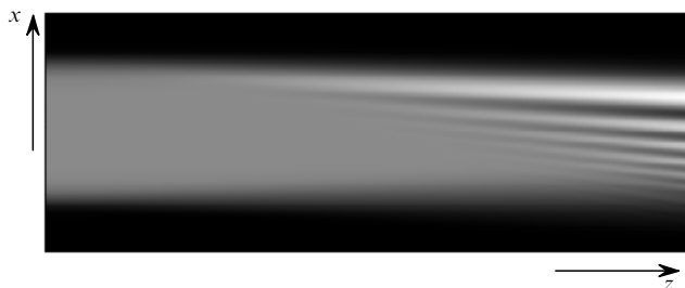
Figure 5. Intensity distribution of the 'rectangular' light beam propagating in a crystal of length 15 mm along the z axis for m = 0.5 , E_m = 5 \text{ kV cm}^{-1} , I_d = 0.01 , and \mu_{\tau} = 2 \times 10^{-12} \text{ m}^2 \text{ V}^{-1} . The scale along the transverse axis x is 14 times enlarged.
