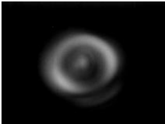
Figure 2. Spatial radiation profile behind the laser spark ( \tau = 110 fs, 80 \text{ J cm}^{-2} ).
