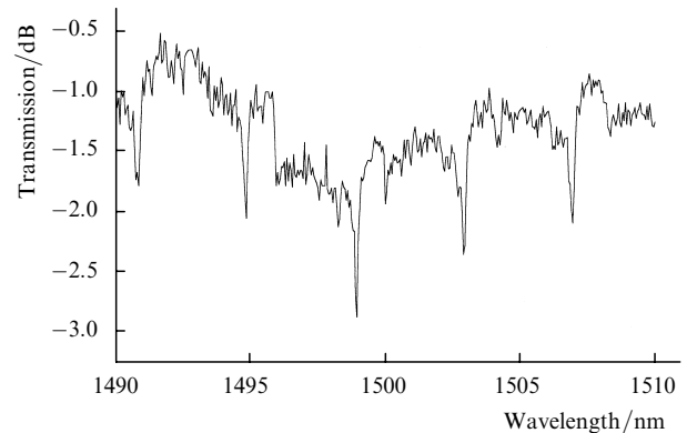
Figure 5. Spectrogram of radiation at the output of a bitapered fibre obtained by exciting WGWs in a standard cylindrical fibre.
