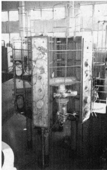
Figure 2. Wide-aperture laser with an active volume of 600 L pumped by 12 electron beams.
