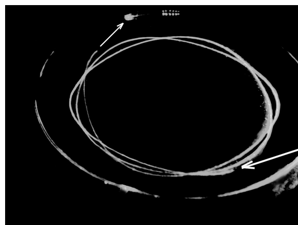
Figure 1. Three-coil track of length 35\ \text{cm} on a concave liquid film of diameter 65\ \text{mm} . The focal point of a 5\text{-mW} cw laser beam on the film surface and the exit of light from the film are shown by the arrows.
