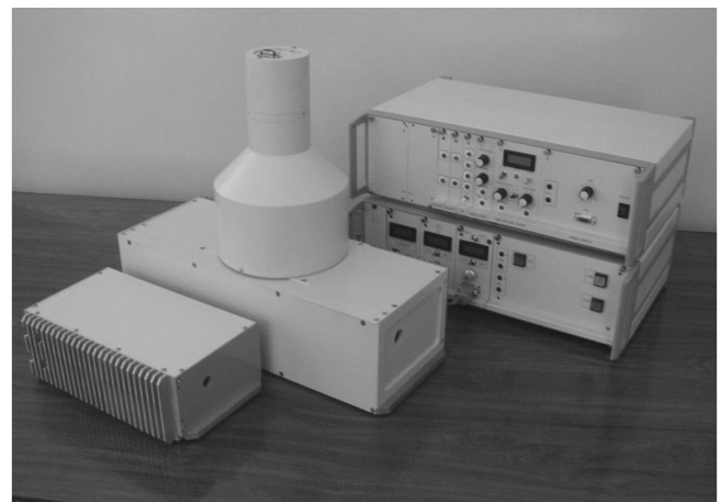
Figure 9. Transportable frequency standard based on the Nd:YAG/I _2 system.
