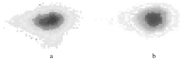
Figure 3. Distributions of the radiation intensity over the beam cross section at the OPO output at an idler-wave frequency ( \lambda = 3.03 \mu\text{m} ) for z = 11 \text{ mm} in the near-field (the distance from the OPO output mirror is 160 \text{ mm} ) (a) and far-field (at the focus of a lens with f = 100 \text{ mm} ) (b) regions.
