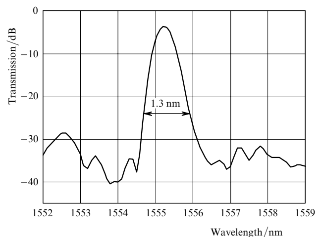
Figure 2. Spectral transmission characteristic of a demultiplexer.
