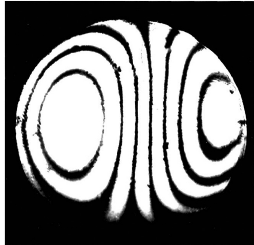
Figure 3. Reverse-shearing interferogram characterising the aberration of the experimental setup.
