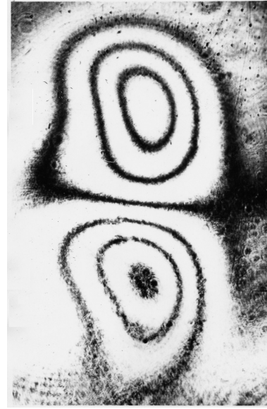
Figure 2. Lateral shear interferogram of a polymethyl methacrylate plate obtained by adjusting to an infinitely broad fringe.
