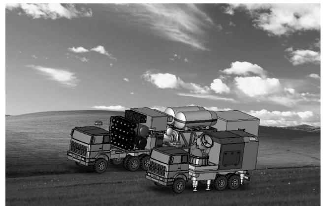
Figure 12. Assembly of a 50-kW COIL with a cryoadsorption recovery system and the beam control system.
