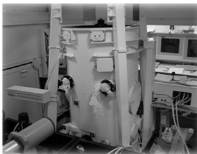
Figure 8. Focusing telescope for the beam control system: (1) main mirror; (2) secondary mirror; (3) refocusing mechanism; (4) telescope casing; (5) tip-tilt mirror; (6) radiation introduction channel; (7) spiders; (8) windows for installation of adjusting elements.
