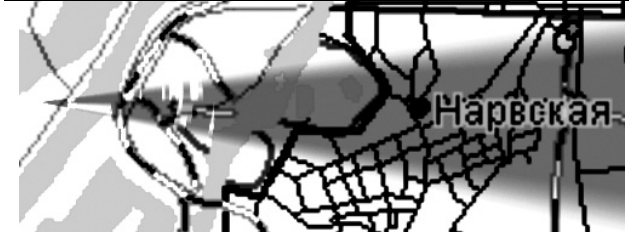
Figure 16. Results of measurement of the background concentrations of \text{NO}_2 in a natural urban landscape of St. Petersburg. The light regions in the probe sector correspond to areas with a concentration exceeding 1 ppm.
