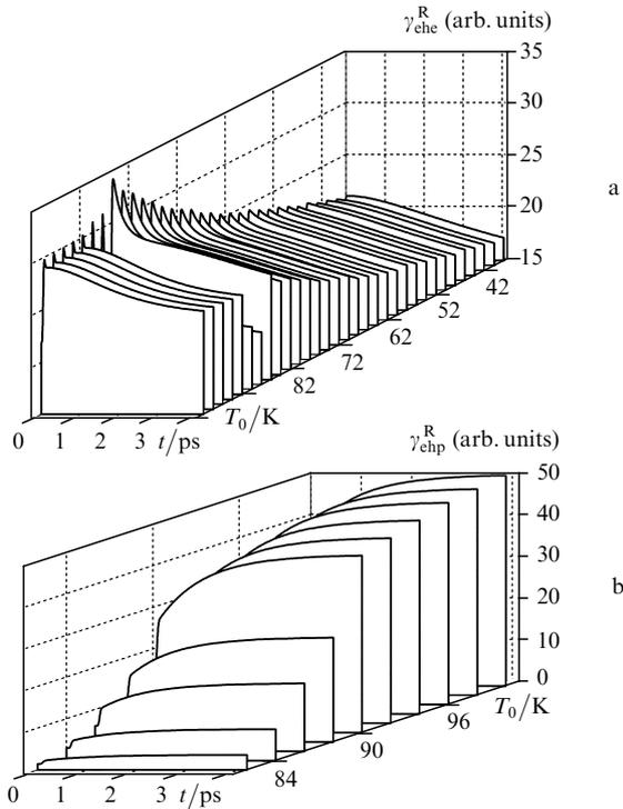
**Figure 3.** Changes in the kinetics of the rates of three-particle recombination  $\gamma_{\text{che}}^R(t)$  (a) and  $\gamma_{\text{chp}}^R$  (b) caused by absorption of the pump pulse upon changing the initial temperature  $T_0$ .
