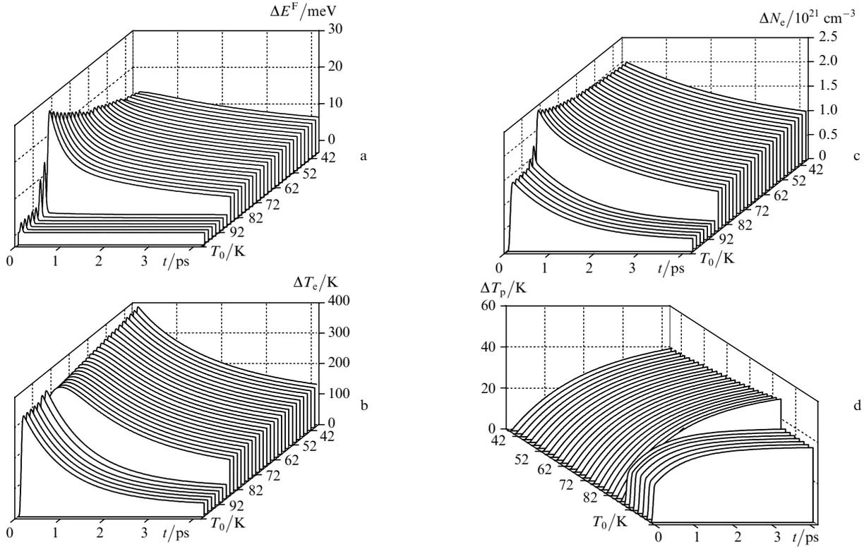
**Figure 2.** Transformation of the kinetics of instant variations in the Fermi level position  $\Delta E^F(t)$  (a), the temperature  $\Delta T_e(t)$  of the electron subsystem (b), the total initial electron concentration  $\Delta N_e(t)$  in the conduction band (c), and the lattice temperature  $\Delta T_p$  (d) caused by the pump pulse upon changing the initial temperature  $T_0$  of the HTSC sample.
