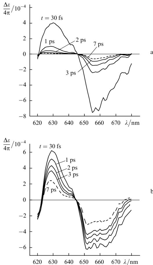
**Figure 5.** Spectral dependences of variations in the modulus of the dielectric constant  $\Delta\epsilon(\lambda)$  of the HTSC sample caused by absorption of the pump pulse upon probing in the wavelength range 620–680 nm at initial temperatures  $T_0 = 100$  (a) and 40 K (b) at different instants.
