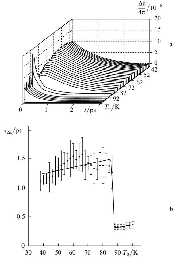
**Figure 4.** Transformation of the kinetics of variations of the modulus of the dielectric constant  $\Delta\varepsilon(t)$  of the HTSC sample caused by the pump pulse upon varying the initial temperatures  $T_0$  (a) and the dependence of the relaxation time  $\tau_{\Delta\varepsilon}$  on  $T_0$  upon probing the sample at the pump wavelength (b).
