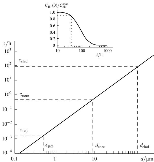
**Figure 1.** Dependence of the characteristic diffusion time  $\tau$  of molecular hydrogen on the silica-cylinder diameter  $d$  at room temperature. The insert shows the dependence of the relative hydrogen concentration on the axis of the fibre of diameter 125  $\mu\text{m}$  on the time after its hydrogen loading.
