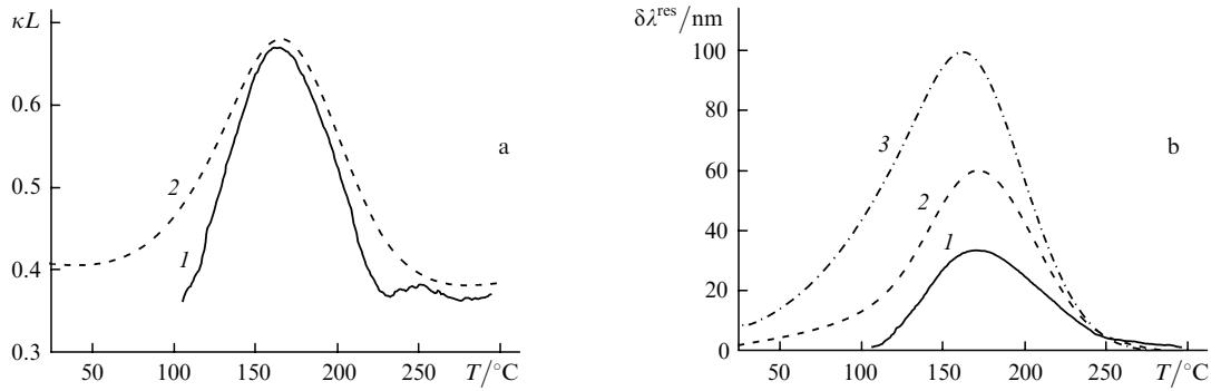
**Figure 7.** Experimental (1) and calculated (2, 3) temperature dependences of  $\kappa L$  (a) and the resonance wavelength shift  $\delta\lambda^{\text{res}}$  (b) for the peak corresponding to the HE<sub>11</sub> – HE<sub>12</sub> mode coupling for a linearly heated fibre. Curve (3) is calculated by (2).
