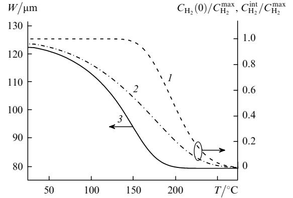
**Figure 5.** Temperature dependences of the relative  $H_2$  concentration on the fibre axis (1), the relative integral  $H_2$  concentration in the fibre (2), and the FWHM  $W$  of the spatial distribution of the  $H_2$  concentration (3) calculated for linear heating of a standard fibre at a rate of  $0.05\text{ }^\circ\text{C s}^{-1}$ .
