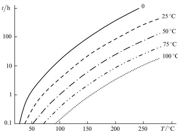
**Figure 8.** Temperature dependences of the hold time of the fibre in the isothermal regime on the temperature upon linear heating at a rate of 0.05 °C s<sup>-1</sup>.
