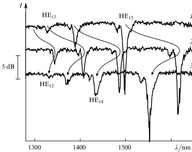
**Figure 2.** Transmission spectra of the LPFG after loading the fibre with hydrogen at temperatures 25 (1), 170 (2), and 300 °C (3) measured during linear heating.
