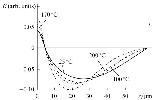
**Figure 6.** Radial distributions of the fields  $E$  of cladding modes  $HE_{12}$  (a) and  $HE_{15}$  (b) calculated at different temperatures upon linear heating of the LPFG in the hydrogen-loaded fibre.
