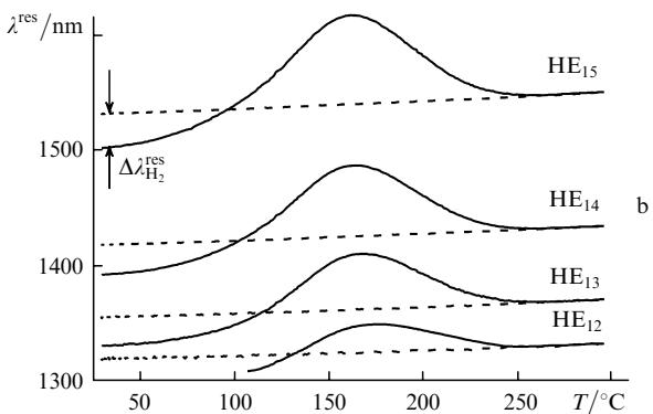
**Figure 3.** Temperature dependences of  $\kappa L$  (a) and the resonance wavelengths  $\lambda^{\text{res}}$  (b) of the LPFG upon linear heating of the grating in the hydrogen-loaded fibre (solid curves) and in the absence of hydrogen in the glass matrix (dashed curves) for different modes.
