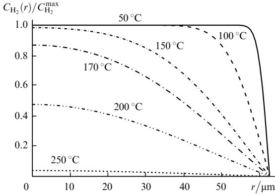
**Figure 4.** Radial distributions of the relative  $H_2$  concentration calculated for a linear heating of a standard fibre at a rate of  $0.05\text{ }^\circ\text{C s}^{-1}$ .
