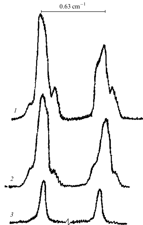
Figure 5. Interferograms of the 546.1-nm laser line of mercury amplified in the dye (1) and injected into the dye (2), and of the He-Ne laser line (3). The line intensities are presented in arbitrary units.
