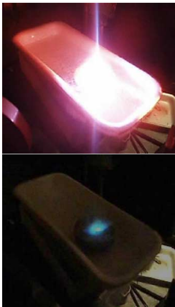
Figure 54. Photographs of emission of the opal surface during the laser pulse (a) and \sim 1 s after the end of the pulse (b).
