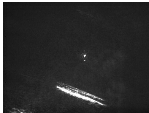
Figure 6. Far-field zones of the distorted and corrected beams with a cylindrical lens aberrator.
