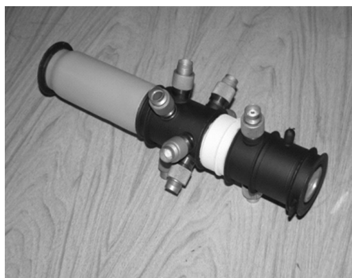
Figure 4. Photoelectron gun with a dynamic focusing lens for time-resolved electron diffraction experiments.
