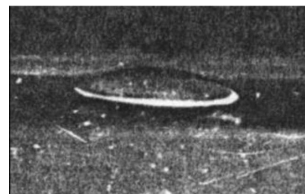
Figure 13. Schematic picture of a geodesic lens ( h_g is the height, R is the radius of curvature, \theta is the polar angle, F = R(1 - \cos \theta)/2 ) (a) and photographs of the lens profile (b) and light beam (top view) focused by the geodesic lens (c).
