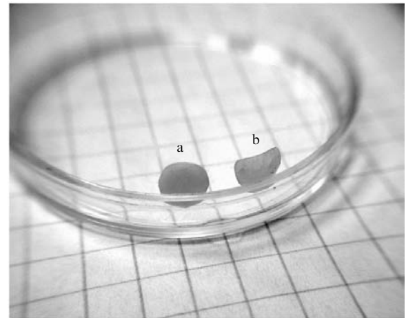
Figure 3. View of a cartilage sample before (a) and after (b) laser irradiation.
