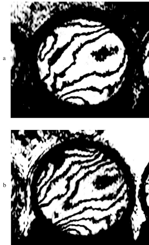
Figure 5. Interference patterns obtained after optical processing of a pair of holographic interferograms located in optically conjugate planes; the measurement sensitivity is higher by 8 (a) and 12 (b) times.
