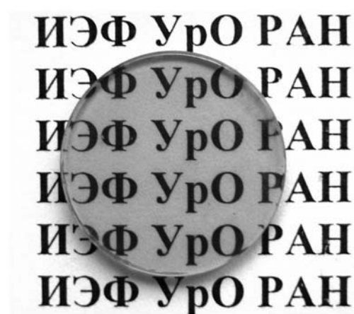
Figure 1. Photograph of a Nd 3+ :Y 2 O 3 ceramic sample with molar concentration of neodymium oxide of 1% [the inscription means IEP, UB, RAS (Institute of Electrophysics, Ural Branch, Russian Academy of Sciences)].
