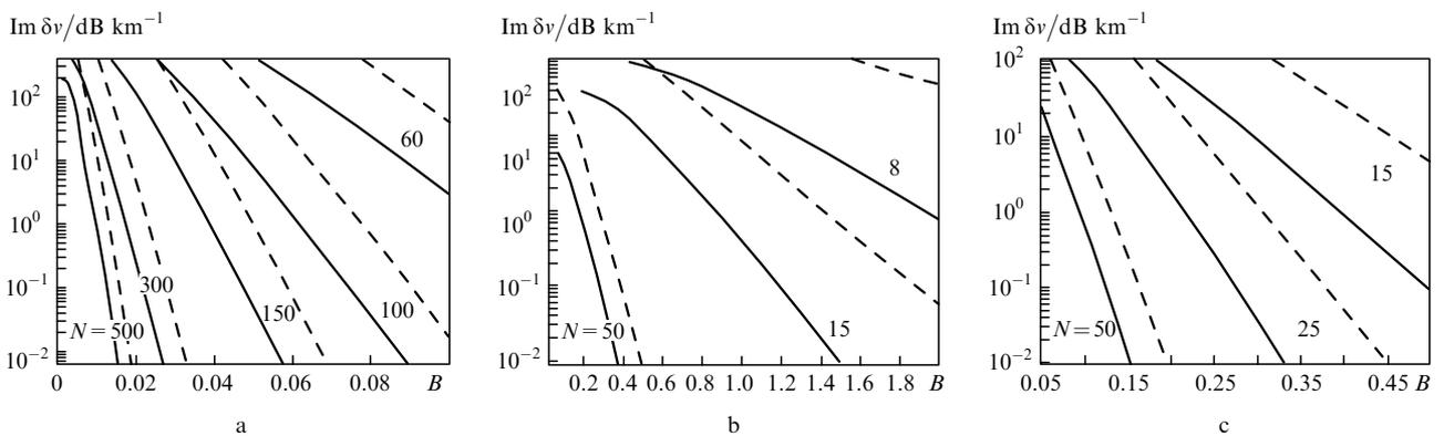
**Figure 8.** Dependence of the radiation losses on the modulation depth of the refractive index for the first (solid curve) and second (dashed curve) modes on the threshold of the third mode appearance for different numbers  $N$  of structure periods and for wavelengths  $\lambda = 1.55$  (a),  $10.6$  (b),  $0.245 \mu\text{m}$  (c);  $\epsilon_1 = 2.6$ , and  $\epsilon = 2.56$ .
