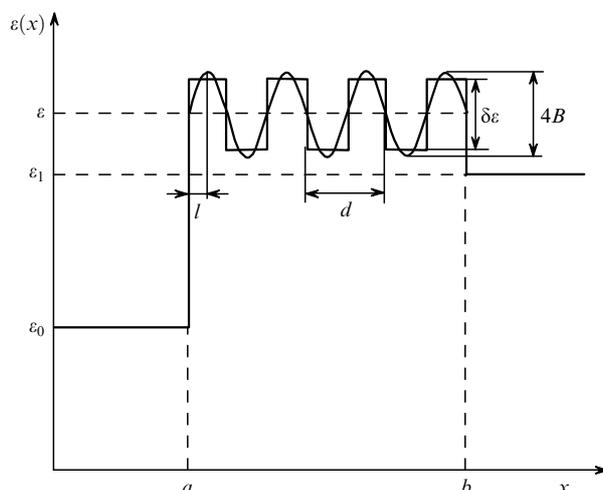
**Figure 1.** Transverse profile of the waveguide permittivity.
