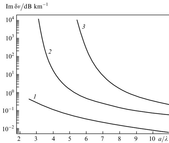
**Figure 7.** Dependence of radiation losses  $\text{Im } \delta\nu$  on the core radius  $a$  normalised to the wavelength; (1, 2, 3) are the mode numbers. Parameters are as in Fig. 6.
