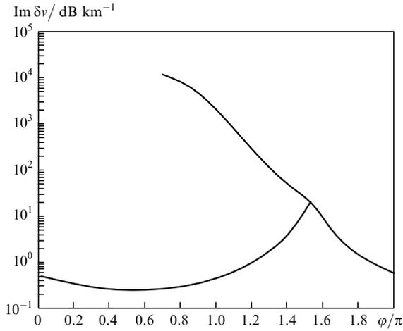
**Figure 6.** Dependence of radiation losses  $\text{Im } \delta\nu$  on the phase  $\varphi$ ; the number of layers is  $N = 150$ ,  $\epsilon_1 = 2.6$ ,  $\epsilon = 2.56$ , and  $B = 0.05$ .
