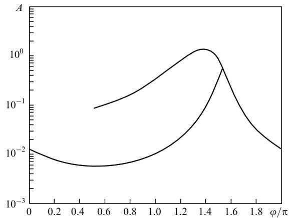
Figure 4. Dependence of the field energy fraction in the cladding  $A$  on the phase  $\varphi$ .
