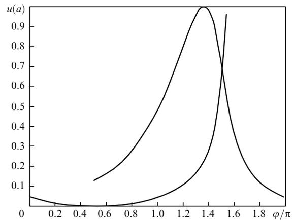
Figure 5. Dependence of the field value at the core-cladding interface  $u(a)$  on the phase  $\varphi$ .
