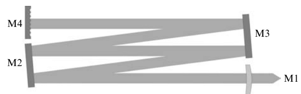
Figure 5. Scheme of the resonator of a industrial CO 2 laser: (M1) ZnSe output mirror with the radius of curvature R = 30 m; (M2, M3) plane folding mirrors; (M4) polarisation-selective element (diffraction mirror or axicon).
