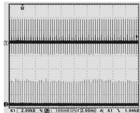
Figure 7. Sequences of the peak discharge voltages ( 2 \text{ kV div}^{-1} ) and the 13.5 \pm 0.135 -nm EUV radiation signals ( 0.52 \text{ mJ mV}^{-1} ) within the solid angle 2\pi sr in the stationary source operation regime at f = 3 kHz.
