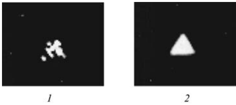
Figure 7. Improved image of a plane triangular rough object obtained by accumulating statistically independent coherent images formed by simultaneous probing the object by several sources: (1) initial coherent object image consisting of seven contrast spots; (2) its improved image formed by accumulating ten statistically independent coherent images.
