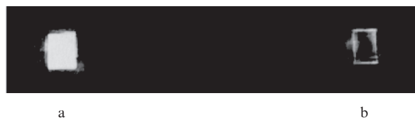
Figure 1. Photograph of a rectangular slit image in the zero diffraction order (a) and its edge obtained in the first diffraction order (b).
