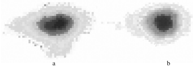
Figure 8. Near-field (the distance from the output OPO mirror is 160 mm) (a) and far-field (at the focus of a lens with a focal length of 100 mm) intensity distributions over the beam section at the OPO output at the idle wave frequency ( \lambda_{\text{idle}} = 3.03 \mu\text{m} ) for z = 11 \text{ mm} .
