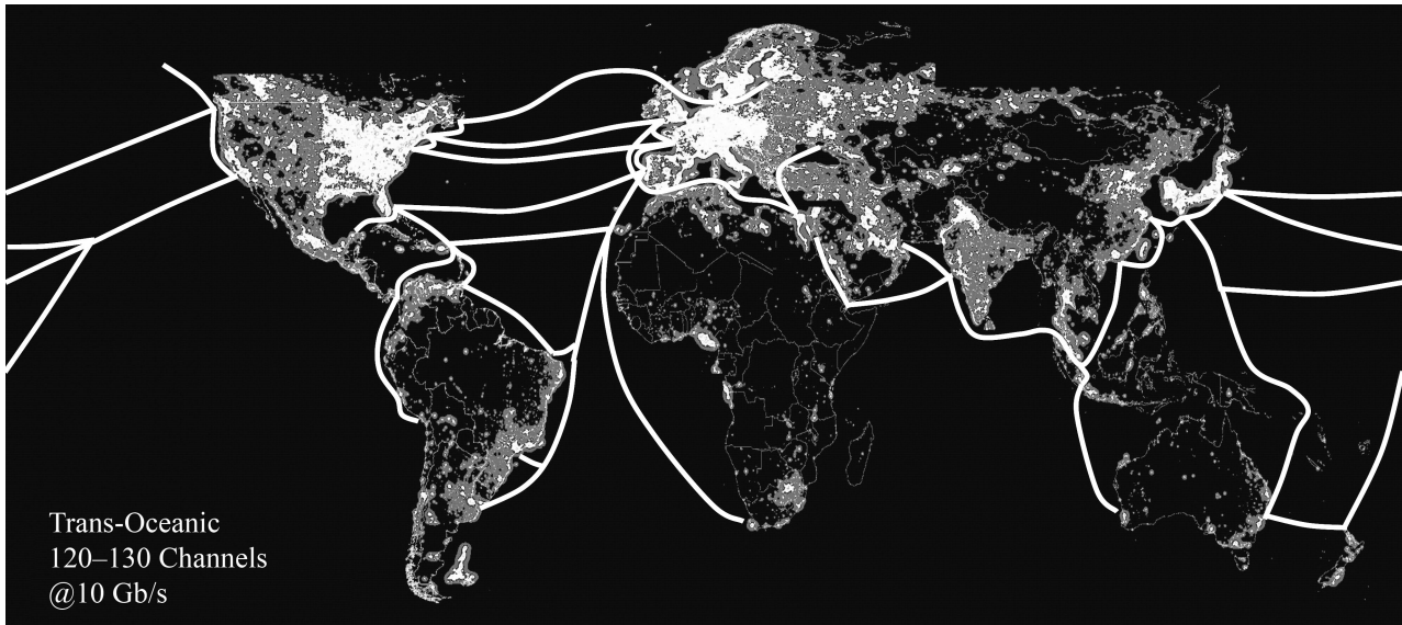
Figure 1. Transoceanic optical fibre communication lines (Alferness R.C., Optical Communications – A View into the Future, Eur. Conf. on Optical Communication, Brussels, 2008).
