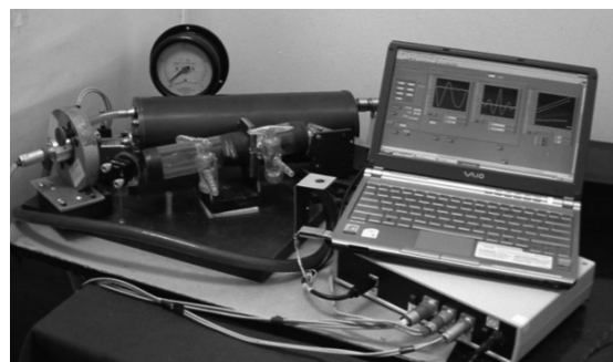
Figure 1. Schematic diagram and photograph of the two-channel DL spectrometer. PD1 and PD2 are photodetectors with preamplifiers in the analytic and the reference channel, the tap and the leak are elements of the vacuum system for gas mixture puffing/evacuation.
