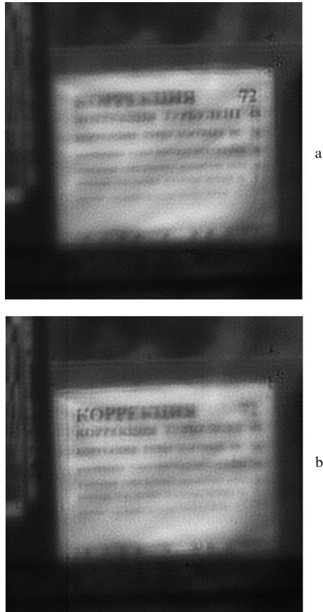
Figure 1. Correction of turbulent image distortions for (a) the number '72' and (b) the letter 'K' in the upper line.
