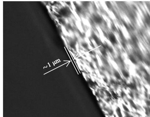
**Figure 5.** Photograph of the sol-gel bonding layer between the YAG crystal and AlN ceramics.
