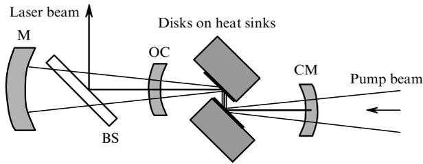
**Figure 6.** Optical setup of lasing experiments with disk elements: (CM) highly reflecting cavity mirror; (OC) output coupler; (BS) beamsplitter; (M) mirror reflecting pump radiation.
