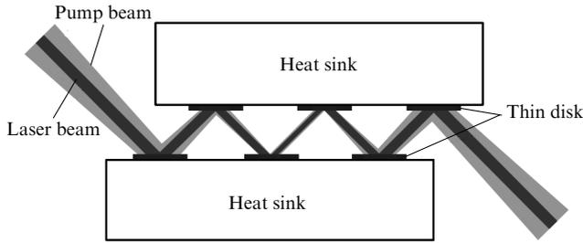
Figure 1. Geometry of collinearly pumped thin multi-disks.
