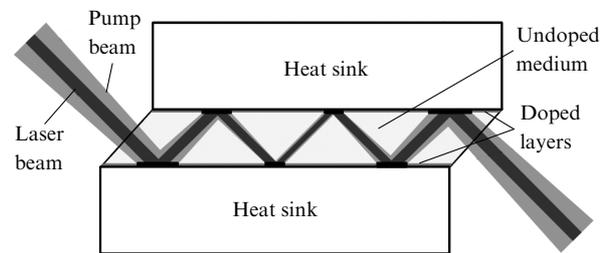
**Figure 8.** Geometry of a composite slab element.
