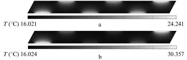
**Figure 10.** Temperature distribution in a composite slab under optimised conditions (a) and twice higher absorption (b). Cooler temperature and pump power are the same for both cases.
