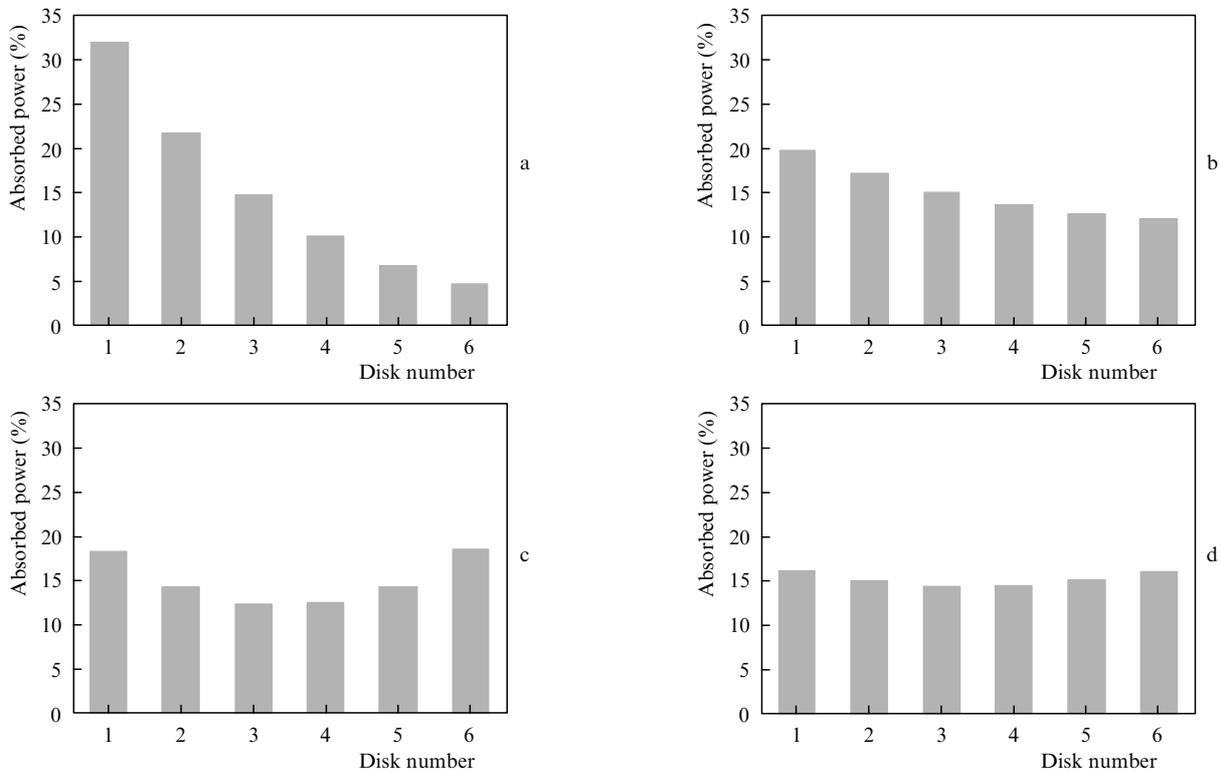
Figure 2. Variation of the absorbed pump power in each disk for different pump schemes: (a) from one end, (b) from one end with residual unabsorbed pump back reflection, (c) from both ends, (d) from both ends with residual unabsorbed pump back reflection. The total absorbed pump power in the structure in each case is 90 %.
