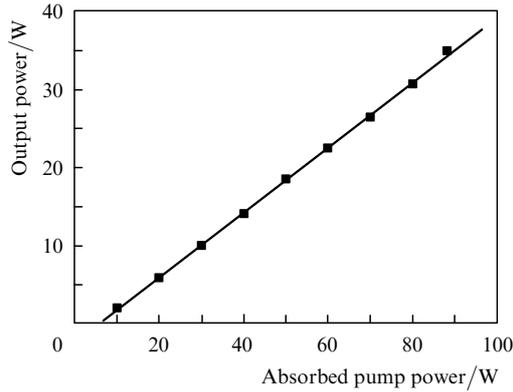
**Figure 9.** Output power versus absorbed pump power for a composite slab geometry.
