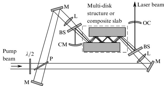
**Figure 3.** Scheme of a two-side pumping configuration with back reflected unabsorbed pump: (M) mirrors; (BS) beamsplitters; (L) lenses; (P) polariser; (CM) cavity mirror; (OC) output coupler;  $\lambda/2$  is the half-wave plate.
