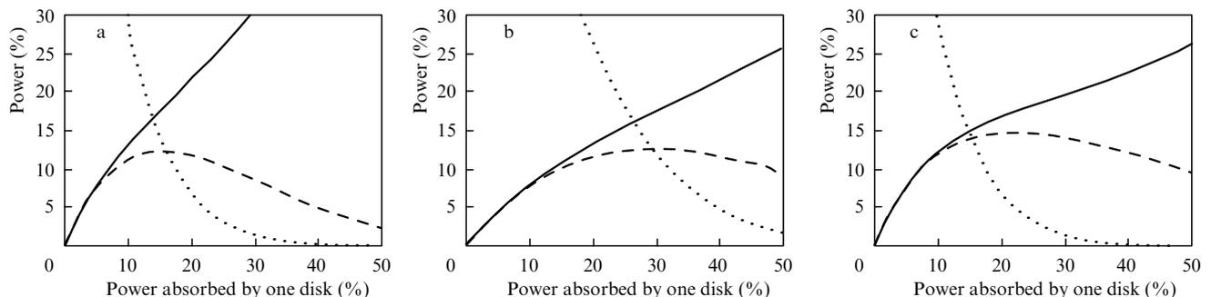
**Figure 4.** Power absorbed in one individual disk versus pump power absorbed in the first disk (solid curves) and in a disk, which absorbs the least power (dashed curves) in the case when (a) the structure is pumped from one side with residual unabsorbed pump back reflection, (b) the structure is pumped from both sides, (c) the structure is pumped from both sides with residual unabsorbed pump back reflection. Dotted curves show the unabsorbed pump in the structure.
