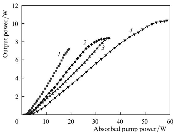
**Figure 7.** Output power versus absorbed pump power for different configurations with disk elements: for (1, 2) one disk and (3, 4) two disks in the case of (1, 3) one-side pumping configuration and (2, 4) one-side pumping configuration with residual unabsorbed pump back reflection.
