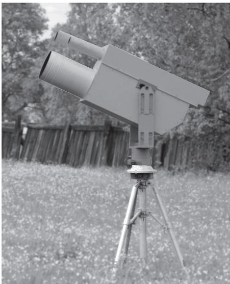
Figure 1. Transceiver of the lidar LOSA-M2.
