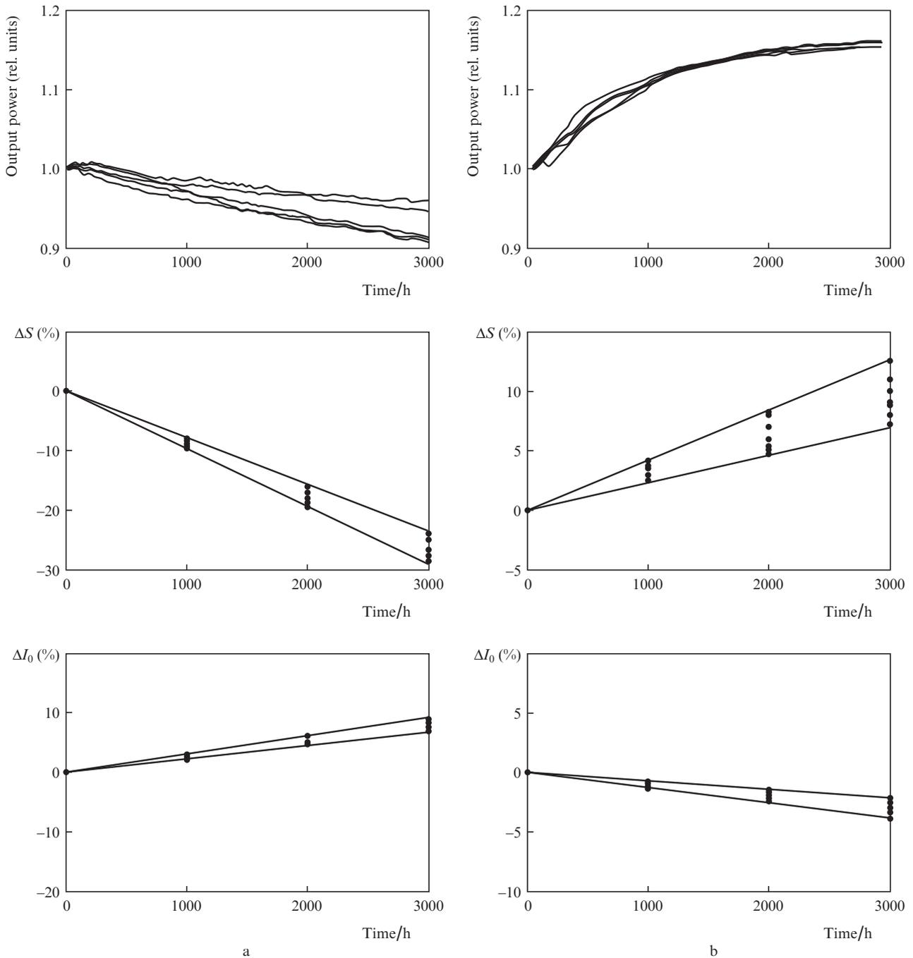
**Figure 4.** Typical dependences  $P_{FS}(t)$ ,  $\Delta S(t)$ , and  $\Delta I_0(t)$  for SLDs of types II–IV (a) and V (b).
