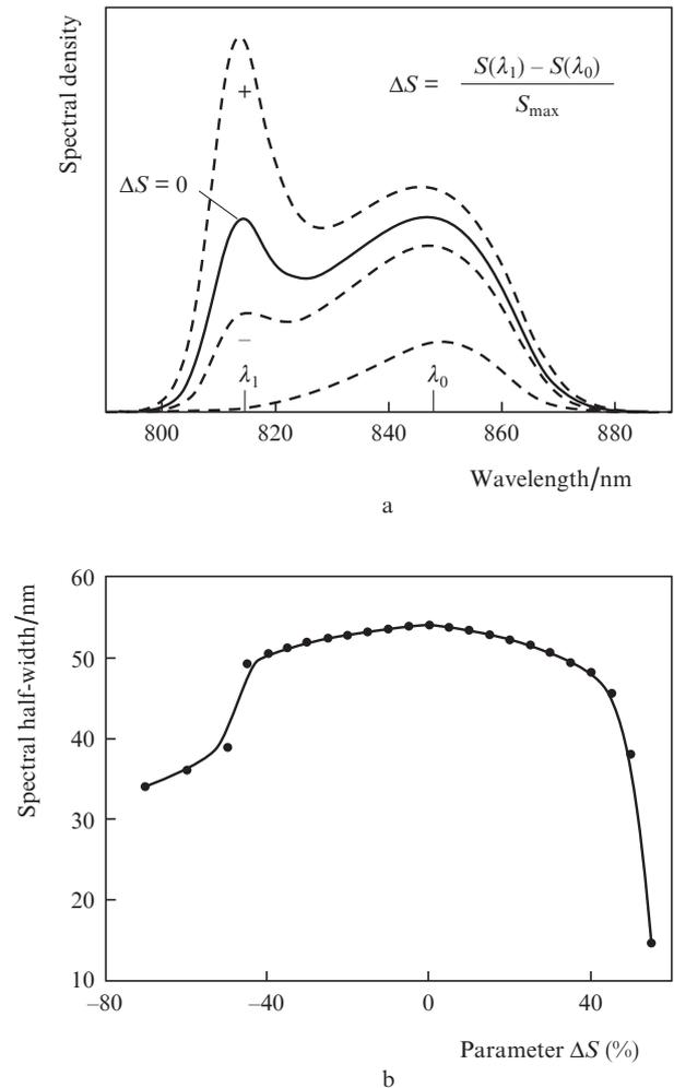
**Figure 1.** Variations in the SLD spectrum with injection current (a) and dependence of the spectral half-width on the  $\Delta S$  parameter (b).
