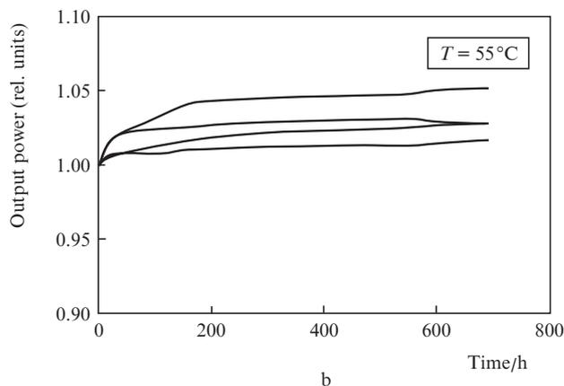
**Figure 3.** Chronograms of the output optical power  $P_{FS}(t)$  of one-type SLDs made of the same PEHS in the ACC regime at 25 and 55°C.
