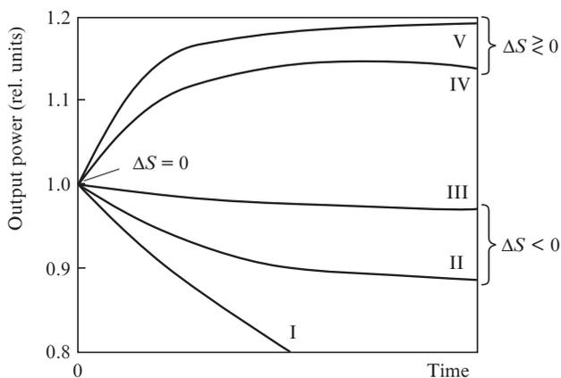
**Figure 2.** Chronograms of the output power for SLDs made of different PEHSs in the course of preliminary life tests in the ACC regime.
