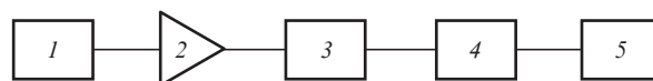
Figure 4. Model of back-to-back line for numerical count: (1) emitter unit, (2) EDFA, (3) tunable dispersion compensator Teraxion, (4) band filter, and (5) optical signal receiver.
