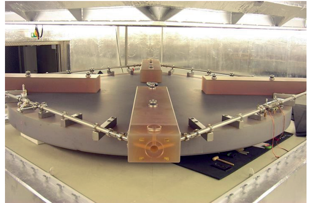
Figure 1. Construction of the G ring laser in the underground laboratory of the Geodetic Observatory in Wettzell (Germany).
