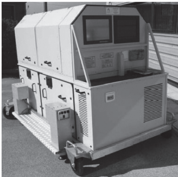
Figure 3. Mobile standoff LIBS system [43].
