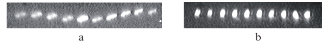
Figure 2. Patterns of the near-field radiation of LD arrays based on AlGaAs (a; nonuniform vertical distribution of emitting elements) and AlGaPAs HSs (b; uniform distribution of emitting elements; near field pattern without smile).
