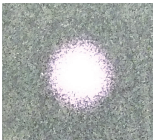
Figure 4. Photograph of graphene luminescence excited by a laser pulse.
