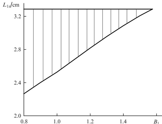
**Figure 2.** Stability region (shaded) in the coordinates  $L_{tr}, B_1$  for the thickness of the nonlinear element,  $L_{dr} = 5$  cm, at the relay telescope length  $L_{tr} = 5$  cm and the refractive index of the nonlinear element  $n = 1.46$ .
