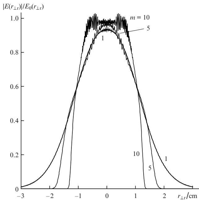
**Figure 3.** Cross sections of the electric field of the laser beam after the 22th stage.
