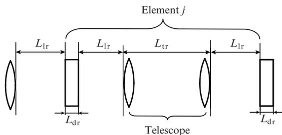
**Figure 1.** Fragment of a transmission line (quasi-optical waveguide) with a relay telescope.
