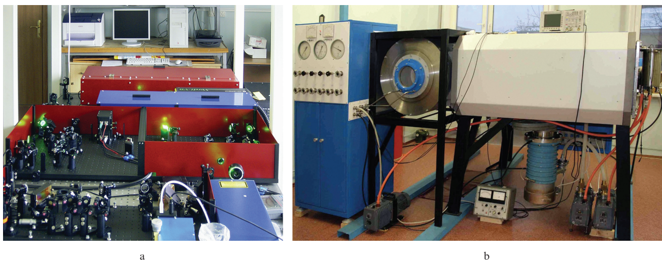
Figure 12. System THL-30: photograph of the front end (a) and XeF(C–A) amplifier (b).
