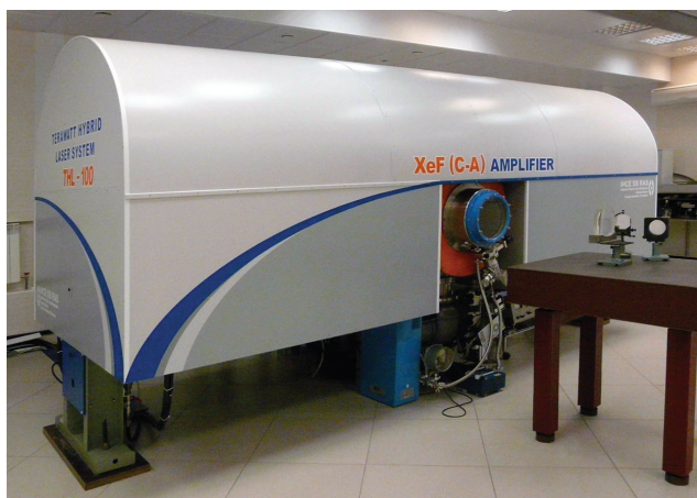
Figure 1. Photograph of a XeF(C–A) amplifier. The overall dimension is 4.5 \times 1.75 \times 1.75 m.
