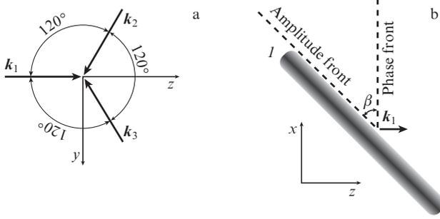
**Figure 1.** Schematic diagram of propagation of linearly polarised laser pulses. The wave vectors  $k_1$ ,  $k_2$ , and  $k_3$  show the directions of propagation of the laser beams in the plane  $(y, z)$  (a). The image of one of the laser pulses ( $l$ ) with the tilted amplitude front ( $\beta$  is the angle between the amplitude and phase fronts) (b).
