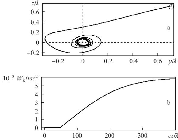
**Figure 3.** 2D trajectory of the electron motion in dimensionless coordinates  $(z/\lambda, y/\lambda)$  (a) and time dependence of the kinetic energy  $W_k/mc^2$  (b) for  $\beta = 45^\circ$ . The parameters of the pulses:  $s = 2$ ,  $ct/\lambda = 3.3$ ,  $\rho_{0\parallel}/\lambda = 200$ ,  $\rho_{0\perp}/\lambda = 2.0$ ,  $I_m/I_{rel} = 1000$ . The coordinates of the initial electron position:  $x_0/\lambda = -10$ ,  $y_0/\lambda = 0.7$ ,  $z_0/\lambda = 0.7$ .
