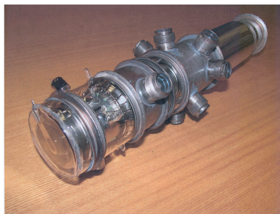
Figure 2. Modified hybrid device ‘ICT–photoelectron gun’.
