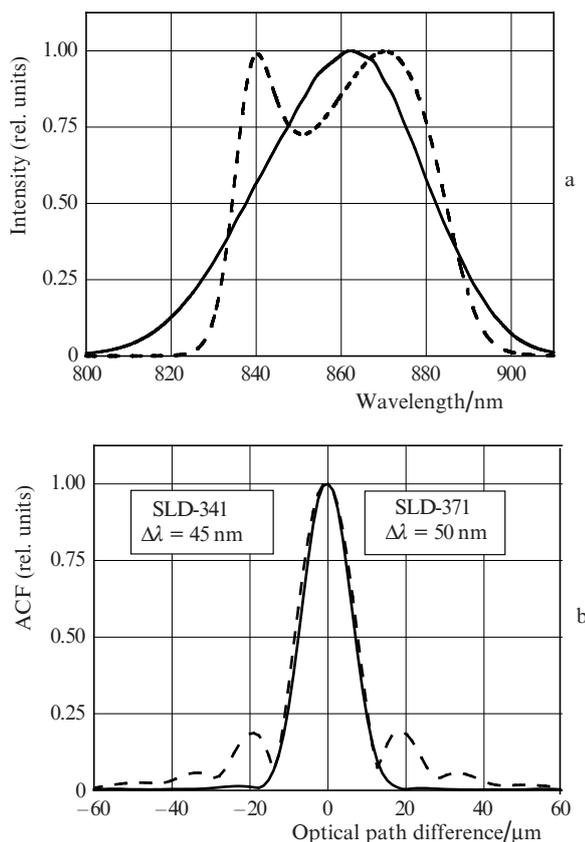
**Figure 7.** (a) Spectra of output radiation and (b) ACF central peaks of the commercial module SLD-371 (dashed curves) and the new module SLD-341 (solid curves).
