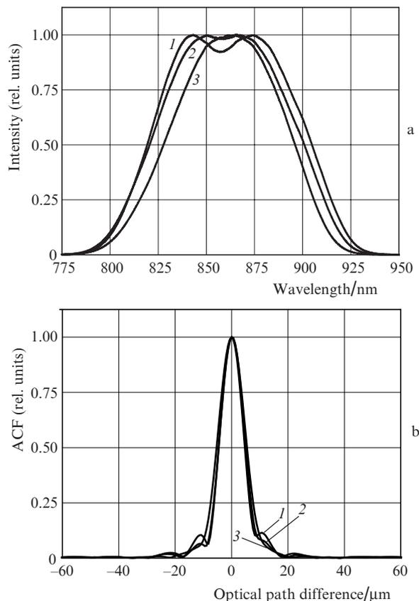
**Figure 8.** Superposition of type II and IV SLD emission spectra in different operation regimes (1–3) (a) and the corresponding ACF peaks (b).
