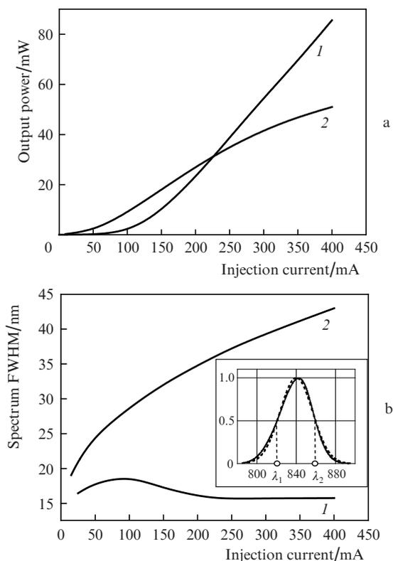
**Figure 2.** (a) Typical light–current characteristics and (b) dependences of the spectrum FWHM on the injection current for (1) the bulk and (2) quantum-well SLDs ( $d_a^{\text{bulk}} = 28$  nm,  $d_a^{\text{SQW}} = 6.5$  nm,  $L_a = 1200$   $\mu\text{m}$ , channel width  $W = 4$   $\mu\text{m}$ ). The inset shows the approximation of the quantum-well SLD spectrum with a Gaussian function (dotted curve).
