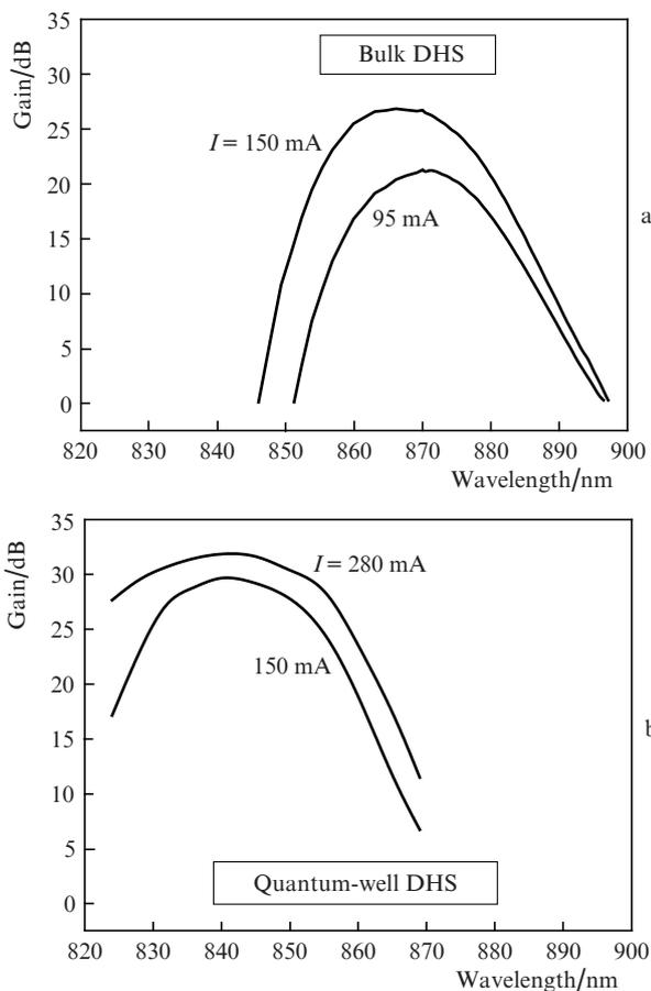
**Figure 3.** Small-signal gain spectra of a SOA on the basis of (a) a bulk ( $L_a = 1200 \mu\text{m}$ ) and (b) quantum-well ( $L_a = 1600 \mu\text{m}$ ) SC DHS.
