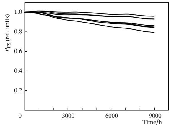
**Figure 6.** Chronogram of lifetest of type II SLDs ( $L_a = 1400 \mu\text{m}$ ,  $P_{\text{FS}} \approx 35 \text{ mW}$ ).
