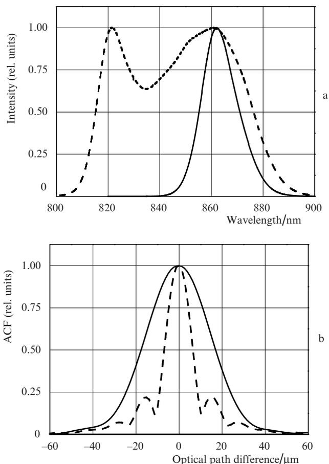
**Figure 1.** (a) Typical spectra and (b) ACF central peaks of the bulk (solid curves) and quantum-well (dashed curves) SLD.
