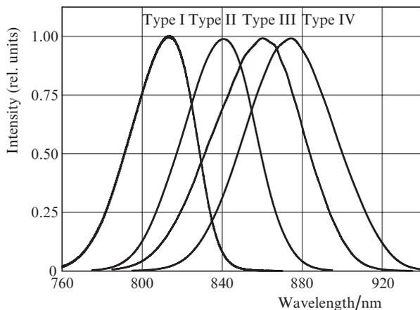
**Figure 5.** Typical emission spectra of the SLD with different composition of the active layer ( $d_a^{\text{SQW}} = 6.0 \text{ nm}$ ).
