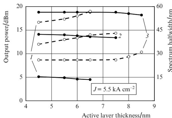
**Figure 4.** Output power (solid curves) and FWHM of the bell-shaped spectrum (dashed curves) vs. the thickness of the active layer for quantum-well SLDs with the median wavelength near 840 nm at  $L_a = (1) 700, (2) 1100$  and  $(3) 1600 \mu\text{m}$ .
