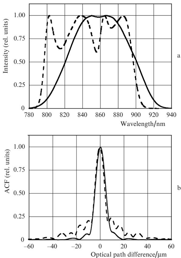
**Figure 9.** (a) Spectra of output radiation and (b) ACF central peaks of the commercial source model BroadLighter D-840-HP (dashed curves) and the new (preliminary D-860-G) model (solid curves).
